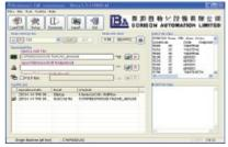
UCAD® universal CAD import and conversion for direct transfer of PCB data from ASCII, AutoCAD and Excel data formats
