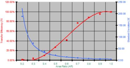
• Transfer Efficiency is the percentage of solder paste of the Theoretical Volume of the aperture that is transferred onto the pad.
